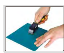
step 1: make grid cutting on surface
