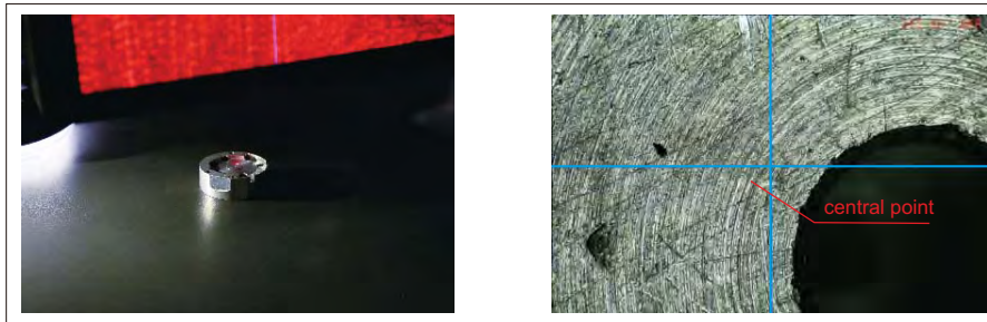
laser indicator locates the central point
