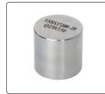
15# carbon steel control sample (optional)
