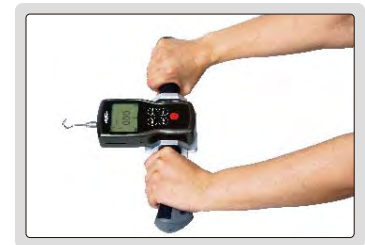
pull test with two handles
