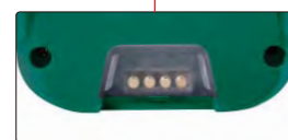
charging and data transmission interface on the back
