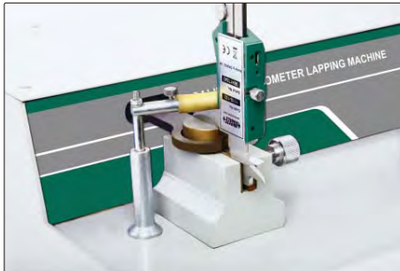
lapping measuring surfaces of caliper lower jaws
