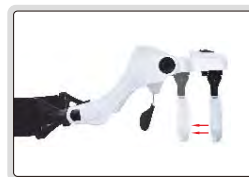
moveable lens for focus
