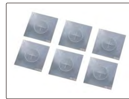
A1 standard sensitivity test piece (optional)
