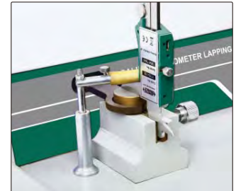
lapping measuring surfaces of caliper lower jaws
